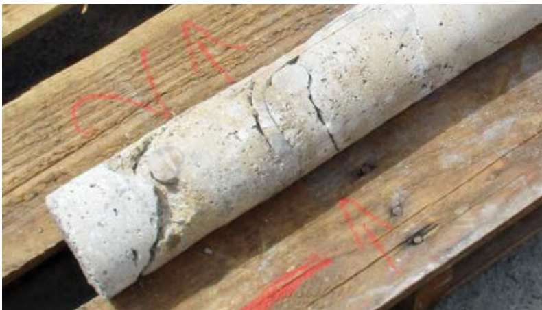
Fig. 7: Irregularities in one of the cores
