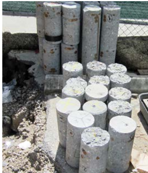
Fig. 4: Cores taken from thick wall preconstruction panels
