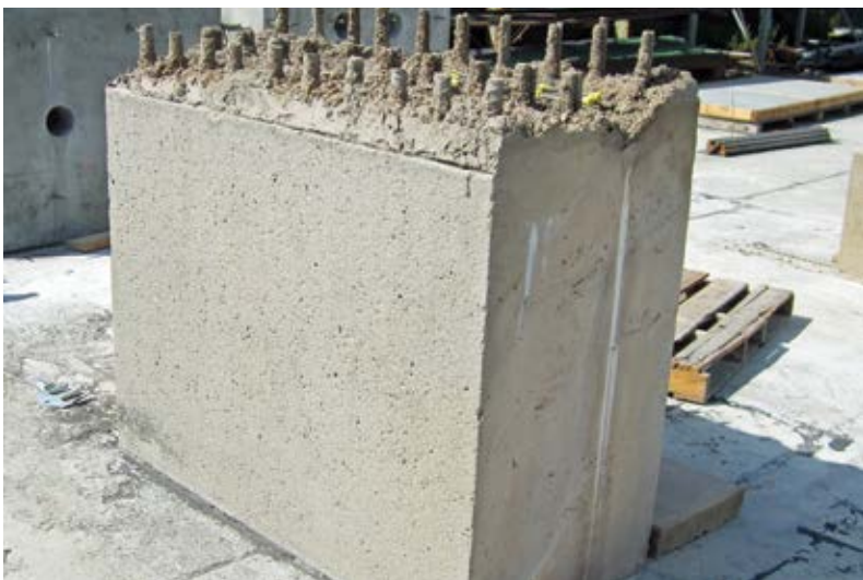
Fig. 8: Lightweight shotcrete mockup panel
